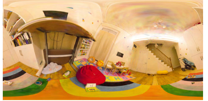
Fig. 14. Complex camera models in radiance fields. We render the playroom dataset (MipNeRF360 datasets [Barron et al. 2022]) using a 360-degree camera. Our ray-tracing-based framework allows us to use arbitrarily complex camera models, as opposed to 3DGS. Artifacts on the ceiling and under the table are due to undersampling in the training data.
