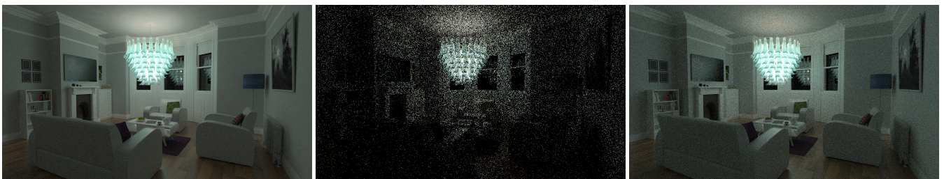
Figure 1: A living room scene containing a learned radiance field-based complex luminaire. From left to right: Reference path-traced scene with explicitly-modeled complex luminaire (32768 samples per pixel, 7.2h); the same scene rendered with 64 samples per pixel in 1.3 minutes; and our method with 32 samples per pixel, 52.1 seconds. We leverage learned volumetric radiance fields to obtain high quality representations of complex luminaires.
