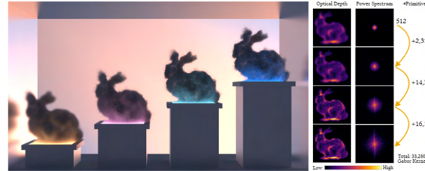
Fig. 1. Example level-of-detail decomposition of our Gabor Fields, a new volumetric density field representation using primitive Gabor kernels. The frequency and orientation-selectivity of the representation enables continuous control over level of detail, reduced rendering time, and a trade-off between variance and bias for performance when sample cost is critical. Here, we show four levels obtained by masking particle collections from the highest-quality asset at render time. (Volumetric Blurry from the OpenVDB database [DuramWorkshopAnimation 2023])
