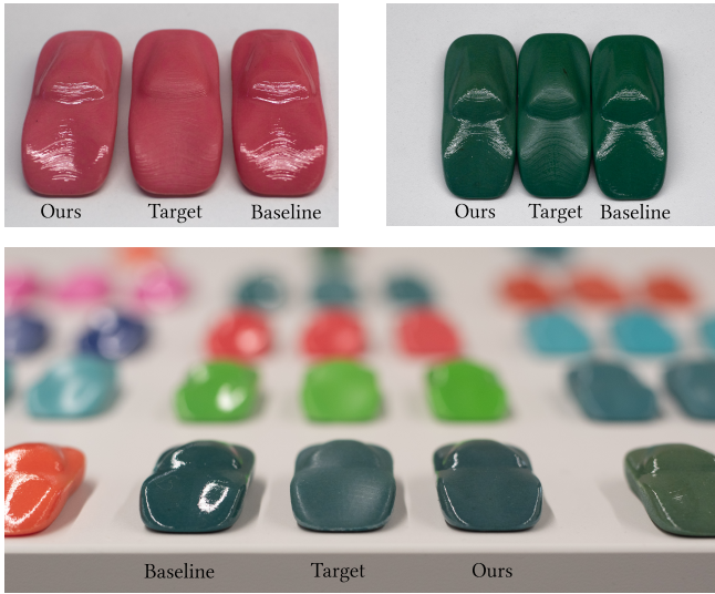
Fig. 9. A small showcase of the color triads presented to test subjects during our experiment in different viewing angles and varnishes (top-left and bottom, Schmincke Matte , top-right, Edding Clear Matte ). Target denotes the target color appearance, while baseline is the same base color on the target surface finish. Ours achieves a closer perceived color to the target, while maintaining the desired glossy surface appearance. Note that due to compression and SDR screen quality, color differences may look substantially smaller than in real life.
